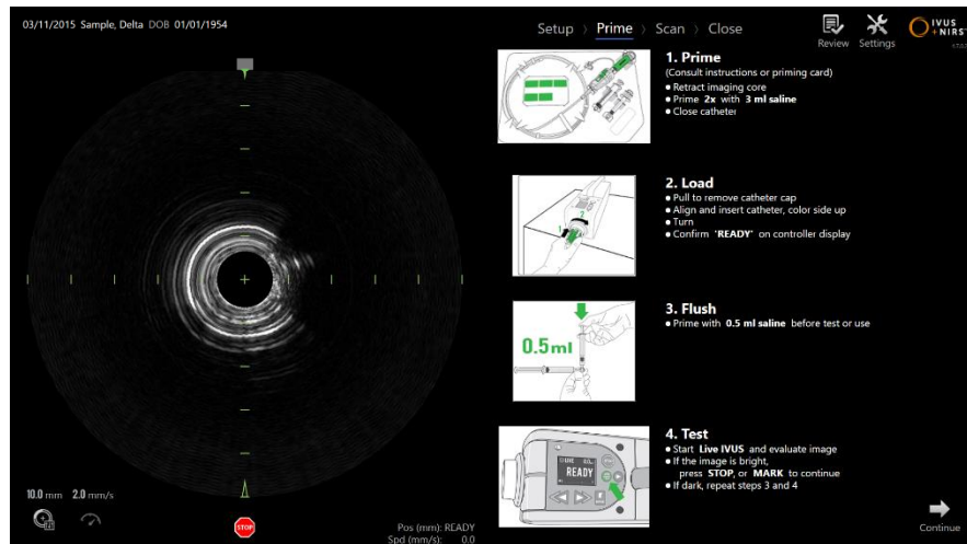
Figure 8-1. Onscreen priming guidance provided in the Prime Phase of Acquisition Mode.
