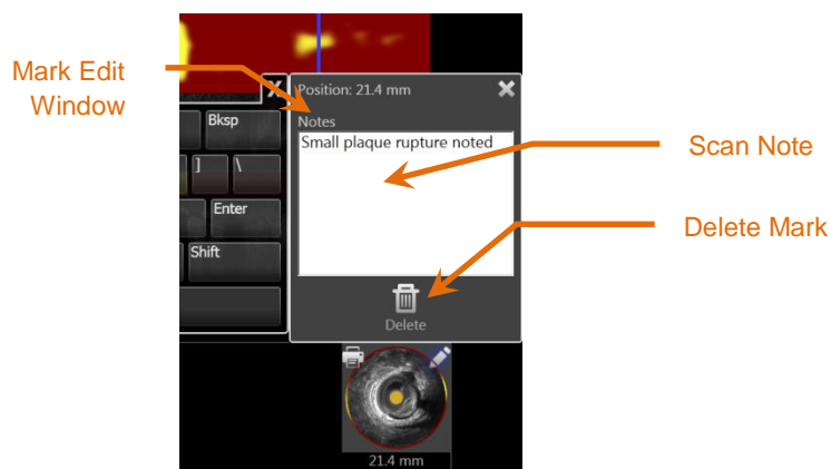
Figure 10-9: Mark Note entered in the Mark Edit Window.
