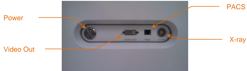
Figure 4-4: Right side interface panel of the Makoto Intravascular Imaging System™ (TVC-MC10) containing the Power Button, Video Out, PACS, and X-ray Integration connectors.
