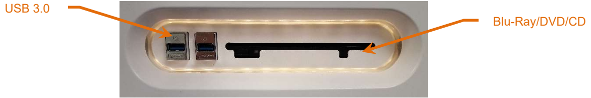
Figure 12-8: Makoto Intravascular Imaging System™ removable media panel
