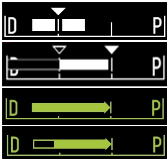
Figure 4-16. Recorded Range during the current acquisition: Live IVUS with current position the same as the start position (top), Recorded Live IVUS with current position proximal to the last Mark press (middle-top), Automated Pullback with no Marks (middle-bottom), Automated Pullback with solid bar indicating recorded range since last Mark (bottom).
