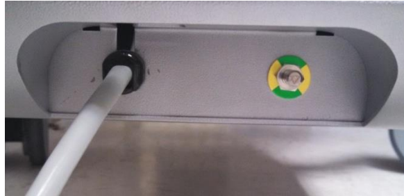
Figure 6-2; Equipotential grounding stud located on the rear of the Makoto Intravascular Imaging System™ on the bottom right edge.
