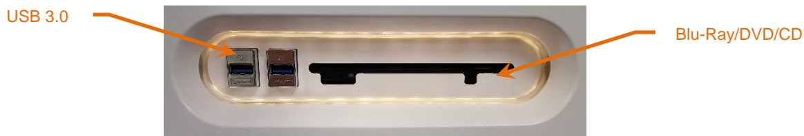
Figure 12-8: Makoto Intravascular Imaging System™ removable media panel
