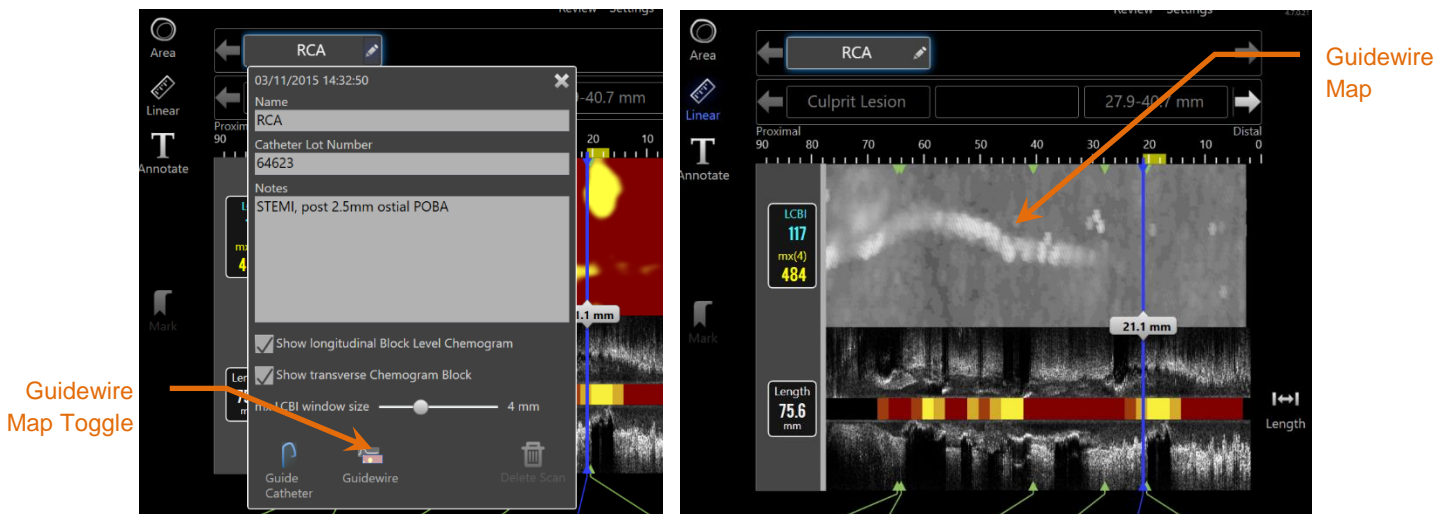
Figure 10-4: Scan Edit window with Guide Wire Map toggle enabled (left); Chemogram is hidden and Guidewire Map is visible (right).
