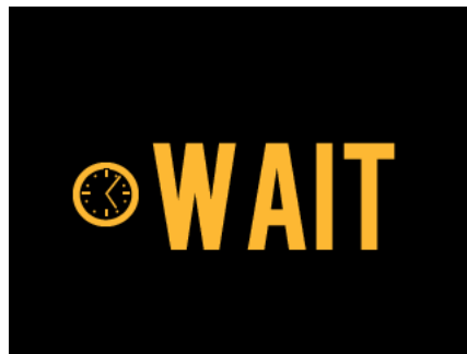
Figure 4-23 The Makoto™ Controller LCD screen indicating a status to wait for the system to complete start up.
