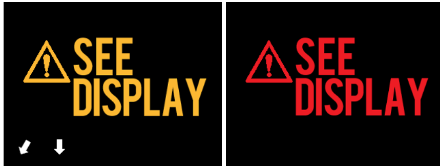
Figure 4-24 The Makoto(tm) Controller error message (left) and internal fault (right) messages. In both cases the user should consult the system monitor for instruction on the error or fault and next actions.
