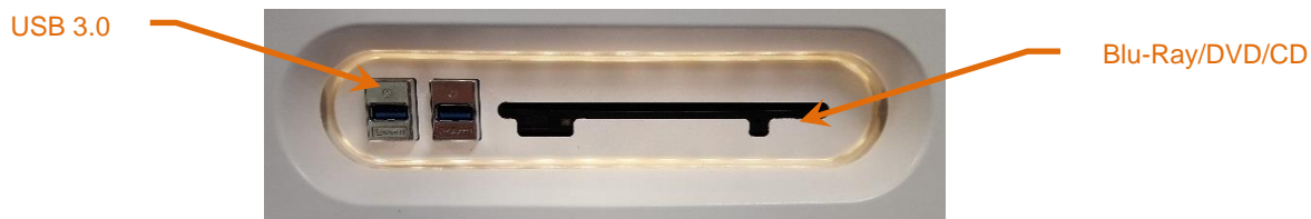
Figur 12-8: Makoto Intravascular Imaging System™ fjernbart mediepanel
