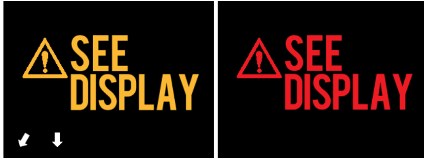
Figure 4-20 The Makoto(tm) Controller error message (left) and internal fault (right) messages. In both cases the user should consult the system monitor for instruction on the error or fault and next actions.
