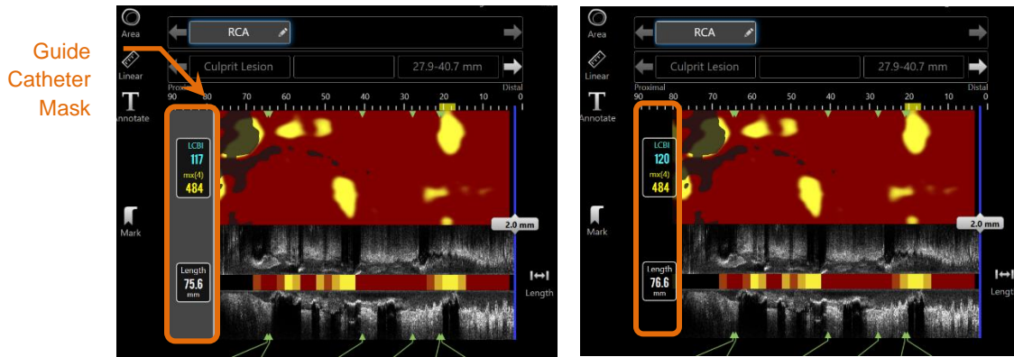
Figure 10-3: Scan Edit with Guide Catheter mask enabled (left). Scan Edit with Guide Catheter mask disabled (right).
