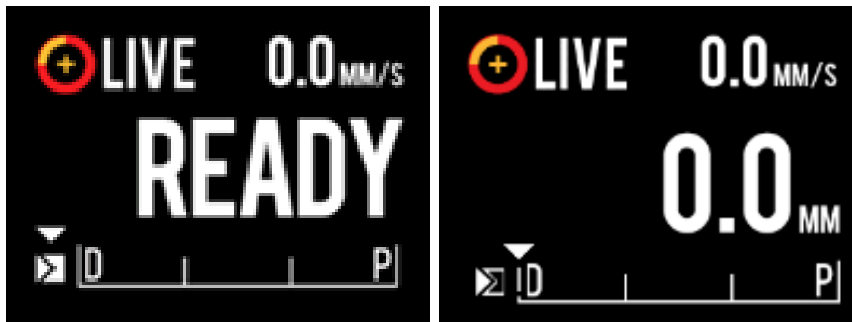
Figure 9-2. Makoto™ Controller with Dualpro IVUS+NIRS catheter connected showing Live IVUS acquisition that is not recorded at the READY position (left) and 0.0 mm position (right).
