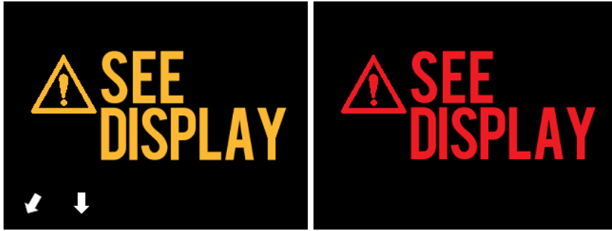
Figure 4-20 The Makoto(tm) Controller error message (left) and internal fault (right) messages. In both cases the user should consult the system monitor for instruction on the error or fault and next actions.
