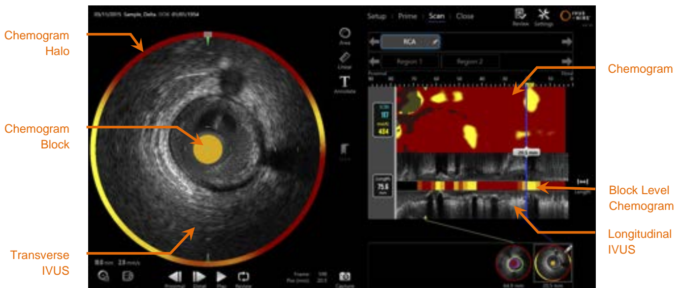
Figure 4-10: Scan Phase of Acquisition Mode with the main displays of image information indicated.
