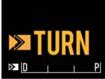
Figure 4-22: The Makoto® Controller LCD screen indicating a instruction to turn the catheter handle.
