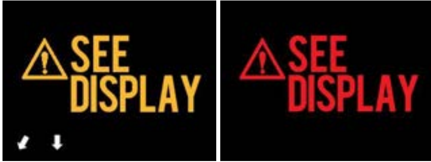
Figure 4-24: The Makoto® Controller error message (left) and internal fault (right) messages. In both cases the user should consult the system monitor for instruction on the error or fault and next actions.
