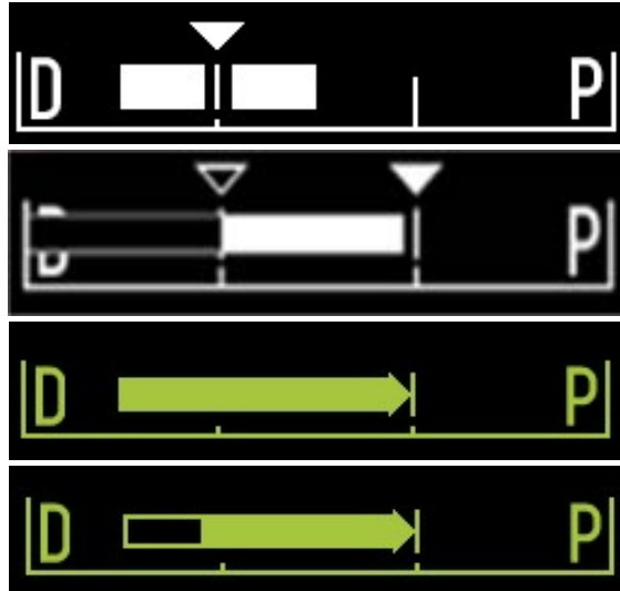
Figure 4-20: Recorded Range during the current acquisition: Live IVUS with current position the same as the start position (top), Recorded Live IVUS with current position proximal to the last Mark press (middle-top), Automated Pullback with no Marks (middle-bottom), Automated Pullback with solid bar indicating recorded range since last Mark (bottom).
