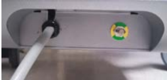
Figure 6-2; Equipotential grounding stud located on the rear of the Makoto® Intravascular Imaging System on the bottom right edge.
