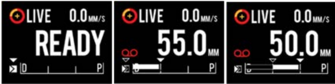
Figure 9-5: Makoto® Controller LCD screen with a IVUS+NIRS Imaging Catheter connected during the process of transitioning from the start of unrecorded Live IVUS at READY (left) to recording then translation proximal and stationary Live IVUS (middle) to zeroing and translating proximal while recording (right). Note the appearance of the recording icon during recorded Live IVUS. When translation is performed during recorded Live IVUS a solid bar appears where the recording in this acquisition was already performed since the last Mark (middle and right) and recording prior to the most recent mark is an empty bar (right).
