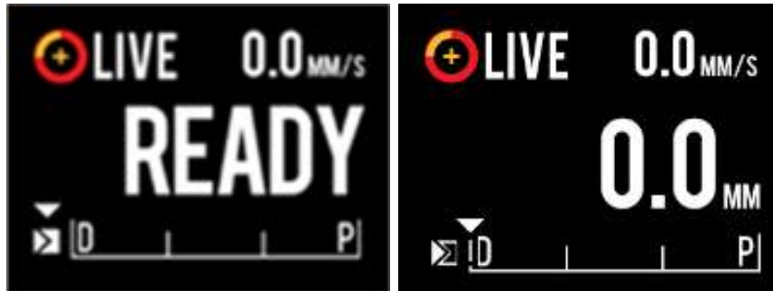
Figure 9-2: Makoto® Controller showing Live IVUS acquisition that is not recorded at the READY position (left) and 0.0 mm position (right).
