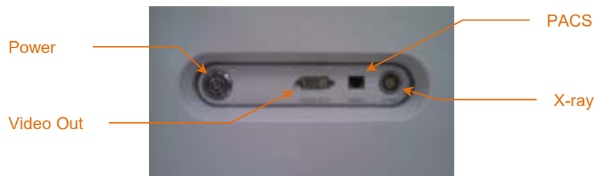
Figure 4-4: Right side interface panel of the Makoto® Intravascular Imaging System (TVC-MC10) containing the Power Button, Video Out, PACS, and X-ray Integration connectors.
