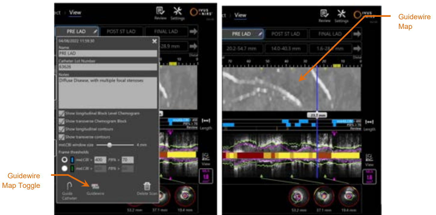
Figure 10-4: Scan Edit window with Guide Wire Map toggle enabled (left); Chemogram is hidden and Guidewire Map is visible (right) (SmartImaging™ optional features enabled).
