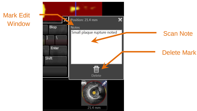
Figure 10-9: Mark Note entered in the Mark Edit Window.
