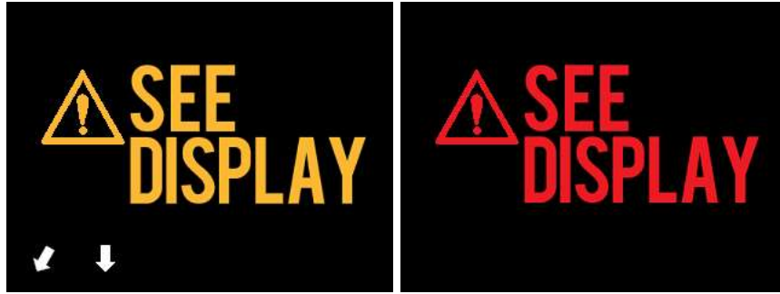
Figure 4-20 The Makoto® Controller error message (left) and internal fault (right) messages. In both cases the user should consult the system monitor for instruction on the error or fault and next actions.
