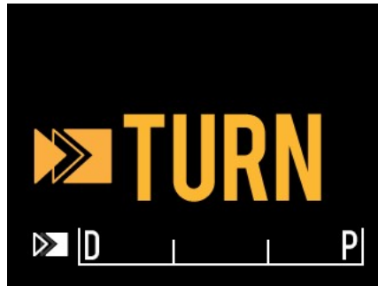
Figure 4-18 The Makoto® Controller LCD screen indicating a instruction to turn the catheter handle.
