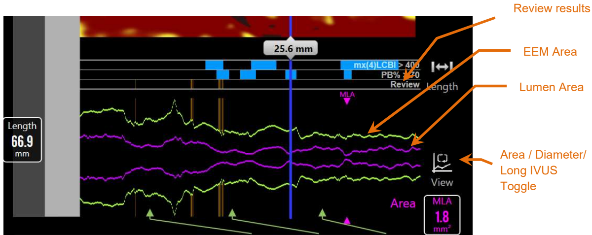
Figure 4-24: Measurement View. Area display shown, the automatically generated EEM area will be presented in green and the lumen area presented in magenta. The corresponding identification will be overlaid on the Longitudinal IVUS display (SmartImaging™ optional features enabled).
