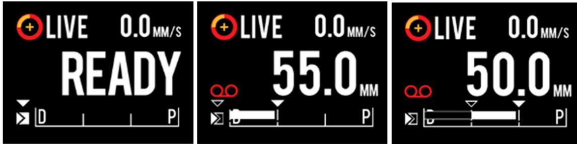
Figure 9-5. Makoto® Controller LCD screen with IVUS+NIRS Imaging Catheter connected during the process of transitioning from the start of unrecorded Live IVUS at READY (left) to recording then translation proximal and stationary Live IVUS (middle) to zeroing and translating proximal while recording (right). Note the appearance of the recording icon during recorded Live IVUS. When translation is performed during recorded Live IVUS a solid bar appears where the recording in this acquisition was already performed since the last Mark (middle and right) and recording prior to the most recent mark is an empty bar (right).
