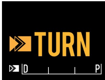
Figure 4-22: The Makoto® Controller LCD screen indicating a instruction to turn the catheter handle.
