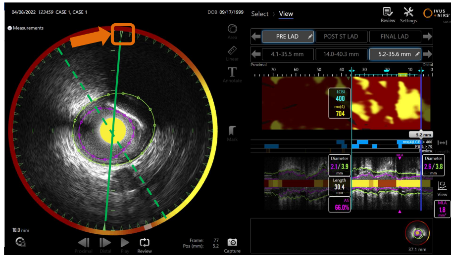
Figure 10-22: Longitudinal IVUS rotation. The dashed green line illustrates where the axis of the longitudinal IVUS started and the solid line illustrates where the axis is currently (SmartImaging™ optional features enabled). The lines are enhanced here for illustrative purpose.
