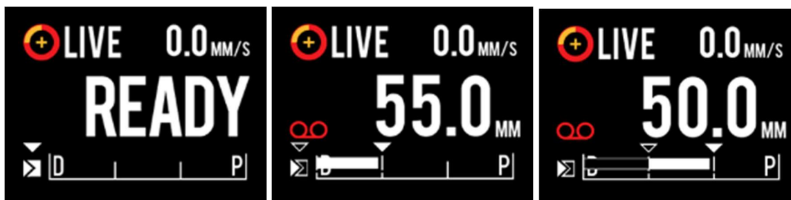
Figure 9-5: Makoto® Controller LCD screen with a IVUS+NIRS Imaging Catheter connected during the process of transitioning from the start of unrecorded Live IVUS at READY (left) to recording then translation proximal and stationary Live IVUS (middle) to zeroing and translating proximal while recording (right). Note the appearance of the recording icon during recorded Live IVUS. When translation is performed during recorded Live IVUS a solid bar appears where the recording in this acquisition was already performed since the last Mark (middle and right) and recording prior to the most recent mark is an empty bar (right).
