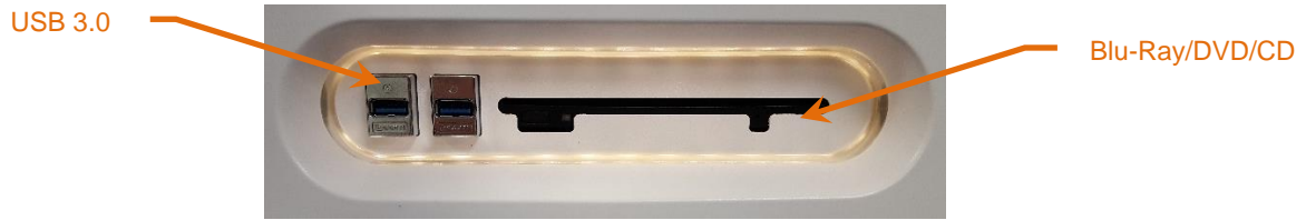
Figure 12-8: Makoto® Intravascular Imaging System removable media panel
